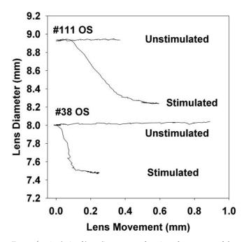
FIGURE 4. Analysis of lens diameter as a function of movement of the center of the circumference of the lens. In two different eyes, EW stimulation produces an accommodative decrease in lens diameter and movements of the lens center (stimulated). Between stimulations, wandering eye movements result in a change in the lens center, but without a change in lens diameter (unstimulated).
