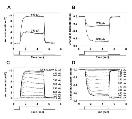
FIGURE 2. Accommodative refractive changes (A, C) and diameter changes (B, D) from monkey 111, left eye. (A, B) Three individual raw traces (essentially superimposed) from three successive stimulations at 250 and 650  $\mu$ A. (C, D) Mean traces covering the full range of responses available to this eye.
